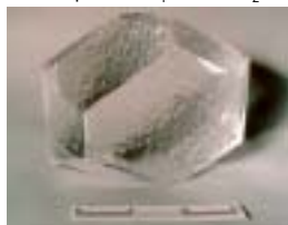
3 inches synthetic quartz crystal for wafer (Fine Crystal Co.)
